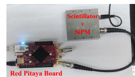
Preliminary Red Pitaya board and scintillator setup
