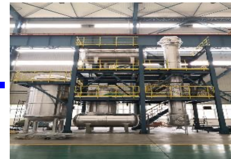
• 3) Water extraction to remove radioactive impurities
