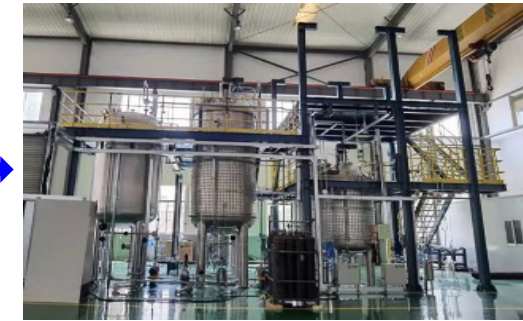
• Mixing LAB with PPO and bis-MSB
